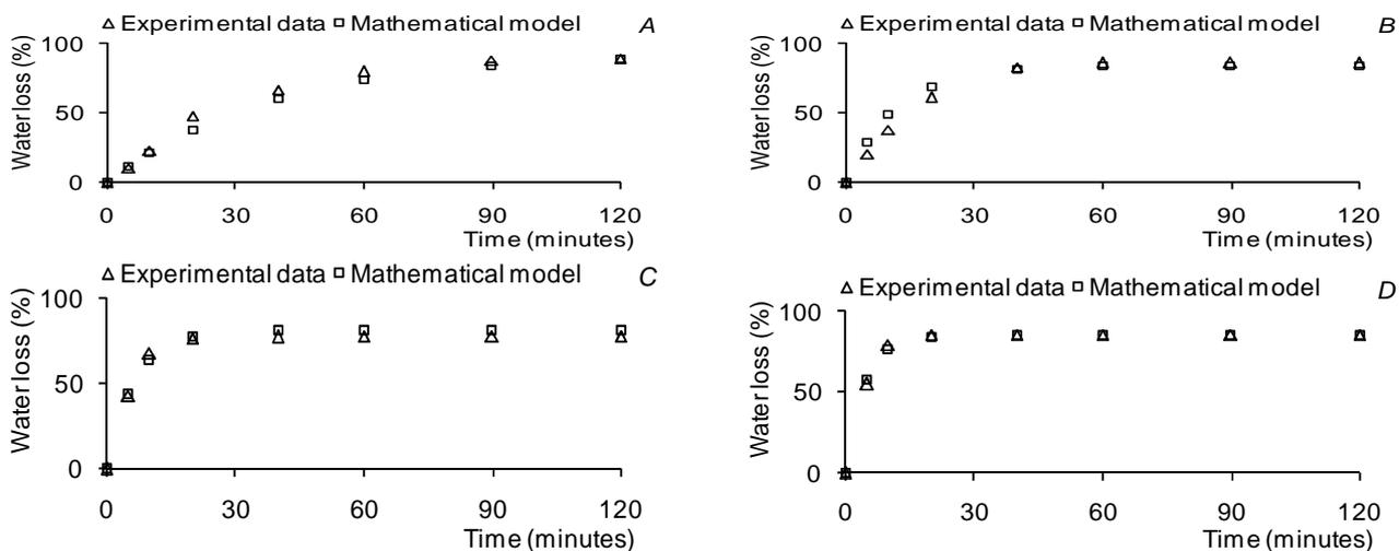
Figure 1. Moisture loss from 5 mm apple cubes during dehydration process at different temperatures (A – 60°C, B – 80°C, C – 100°C, D – 120°C)
