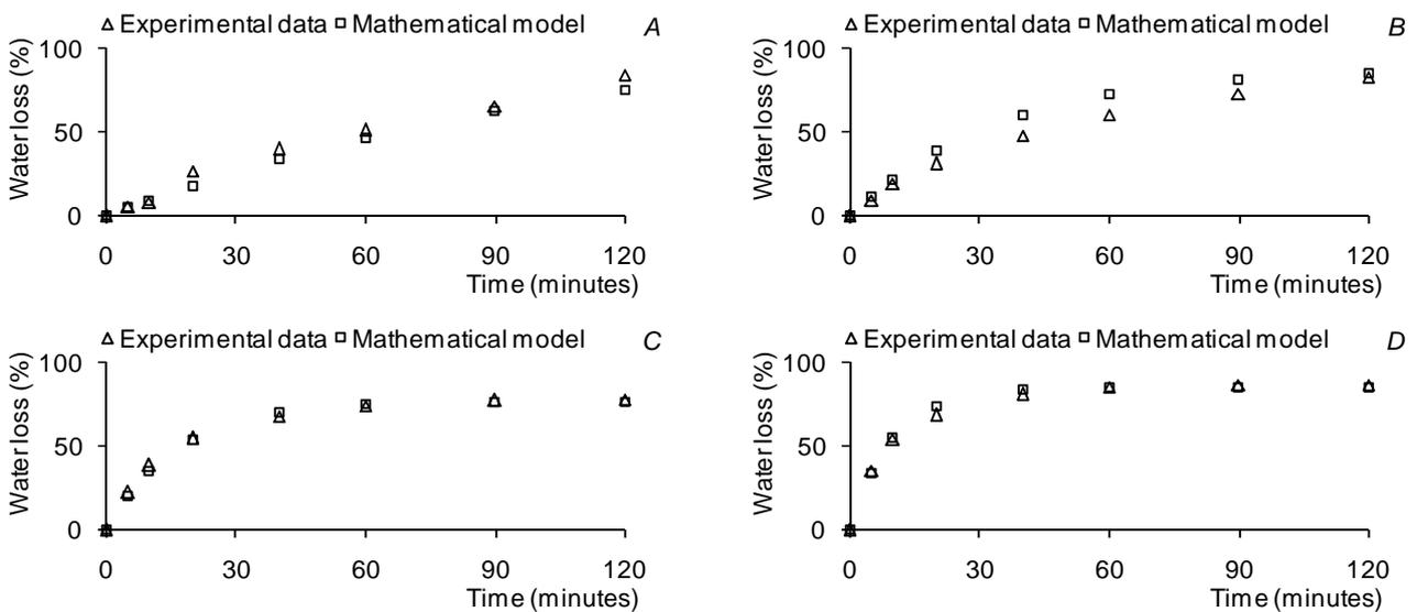
**Figure 3. Moisture loss from 15 mm apple cubes during dehydration process at different temperatures (A – 60°C, B – 80°C, C – 100°C, D – 120°C)**
