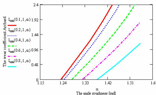
**Figure 4** Variation of the wear coefficient Archard type for the cutting (micro cutting) function of the inclination angle of the roughness
