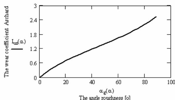
**Figure 3** Variation of the wear coefficient Archard type for plastic deformation function of the inclination angle of the roughness
