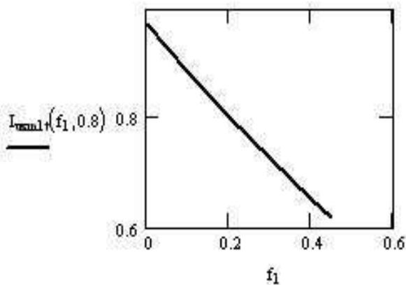
Figure 7 The variation of the medium wear coefficient for an angle  $\alpha_{min} < \alpha < \pi/2$  from which the cutting (micro cutting) appears
