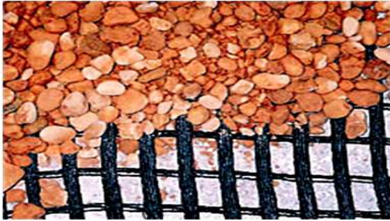
Figure 2 Example of reinforced soil using geosynthetic
